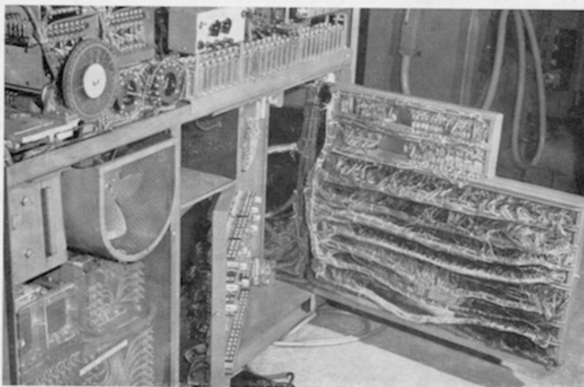
A view of the interior of the Electronic Calculating Punch.
