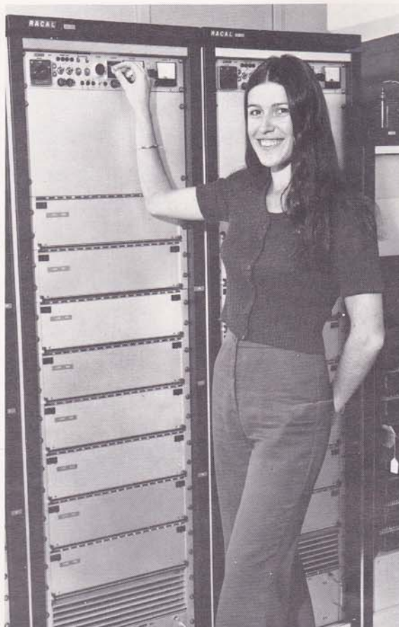
● NEW "HARDWARE". Jenny Hair, of E.D.P. Planning Department, pictured with one of the new items of computer hardware in E.D.P. Operations Department — a line terminating unit which has been described as a "glorified modulating, demodulating unit".
