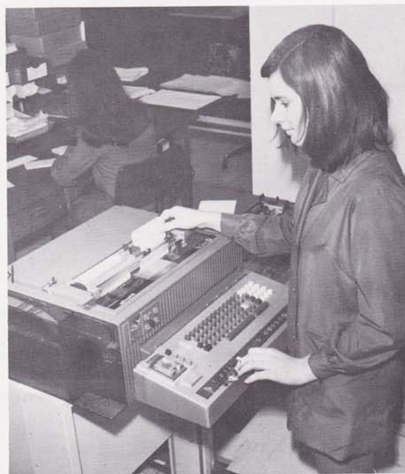
ON-LINE TELLER TERMINAL: This is one of the prototype Olivetti teller terminal machines now being tested at head office. A bandit alarm is built into the mechanism to transmit automatic signals to head office computers. These terminals cost some $4000 each — approximately the same as Sensimatic teller machines. The operator in this picture is Helen Matlik of E.D.P. Operations.
