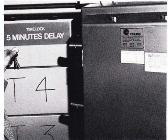
Time locks make it impossible to open a safe cash compartment until a pre-determined period has elapsed after turning the normal key.
